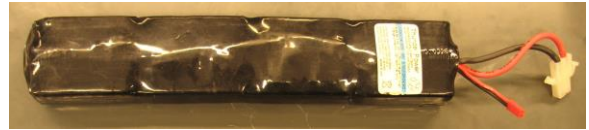
Figure 7: Lithium Polymer Battery
