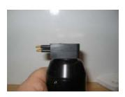
In the 2004 competition Charybdis's center thruster control chip was damaged by water in a pierced cable. To prevent future leakage, all thruster end caps were upgraded with bulkhead connectors to guarantee full water blockage. Micro connectors were used on the thrusters and the electronics tube end cap to reduce the space consumed by connectors. A backup thruster was also acquired as a spare, as our platform depends on all four thrusters being operational for total control.
